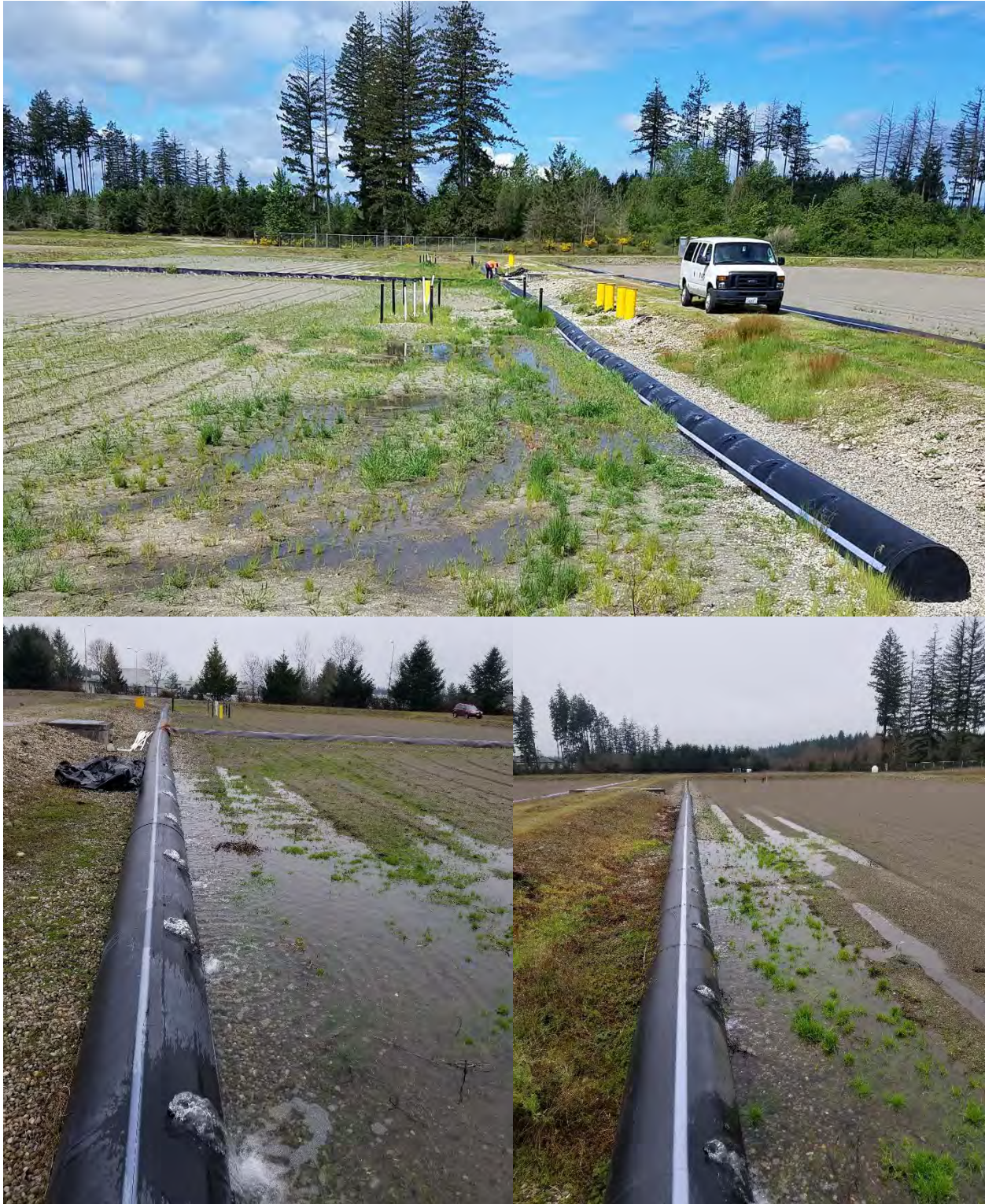
Figure 3-2. Infiltration at Basin 4 during the Tracer Test
