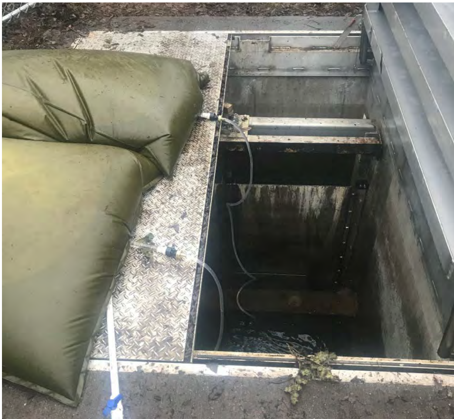
Figure 5-1. Delivery of Bromide (top; tanks) and SF 6 (bottom; bags) Tracers 1/17/2018
