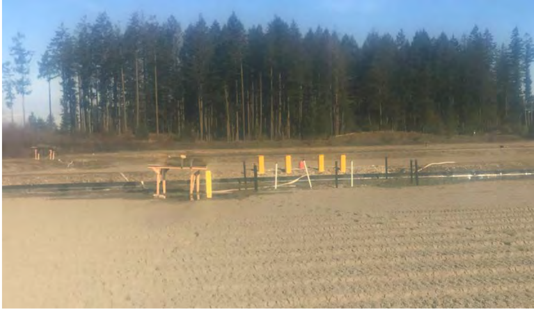
Figure 5-2. Delivery of SF 6 Directly into MW-15 (foreground) and MW-7 (upper left)
