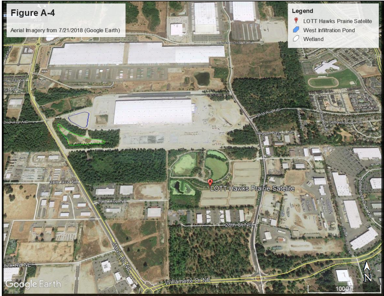
Figure A-4. Estimation of west infiltration pond area (outlined above in blue) and wetland area (above in green). Aerial Imagery from 7/21/2018 (Google Earth).
