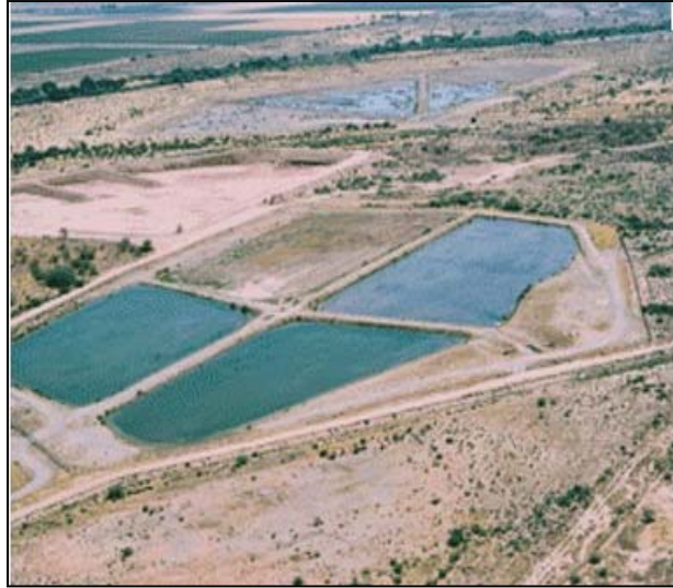
Figure 4-4. Recharge Basin Wetting Cycle
