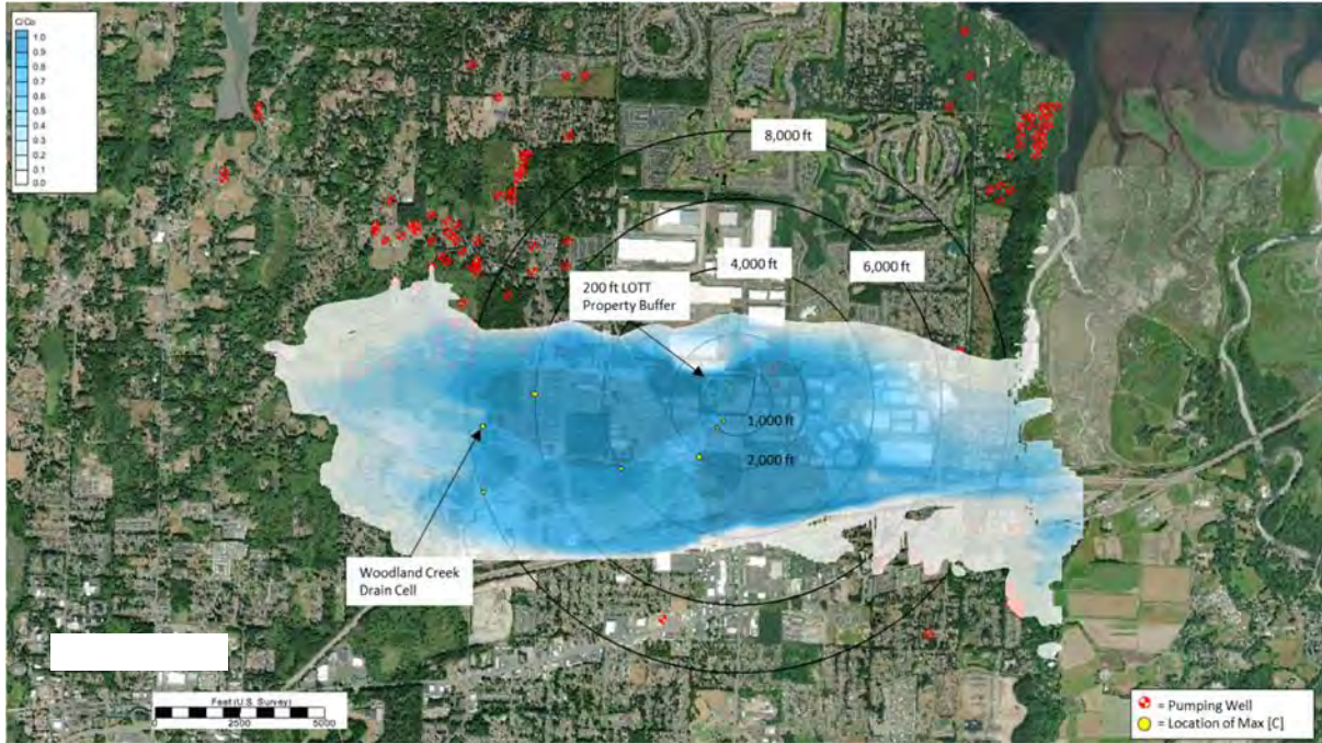
Figure 3 C/C 0 Distribution in the Shallow Aquifer after 100 years
