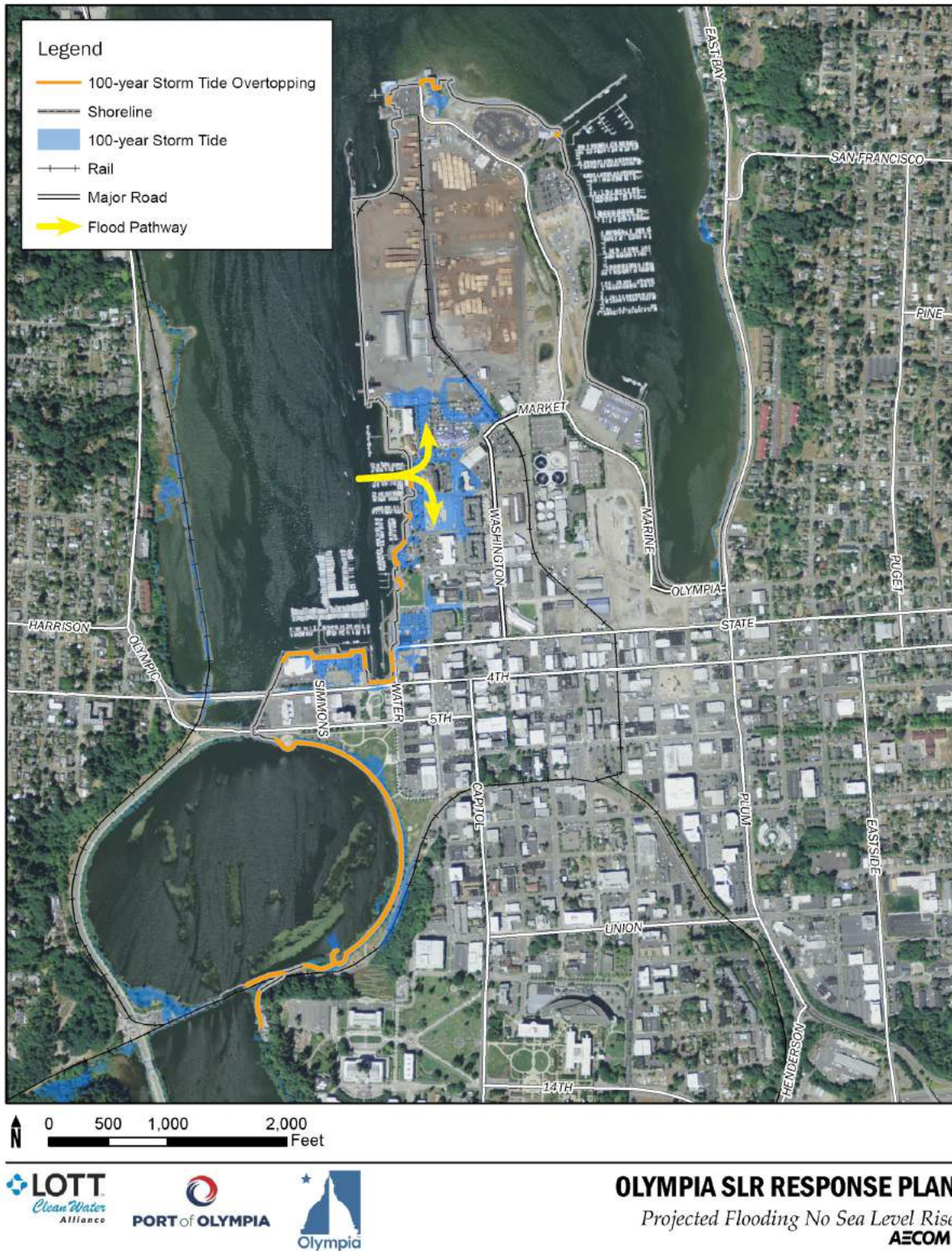
Figure 8. Inundated Assets at No Sea Level Rise
