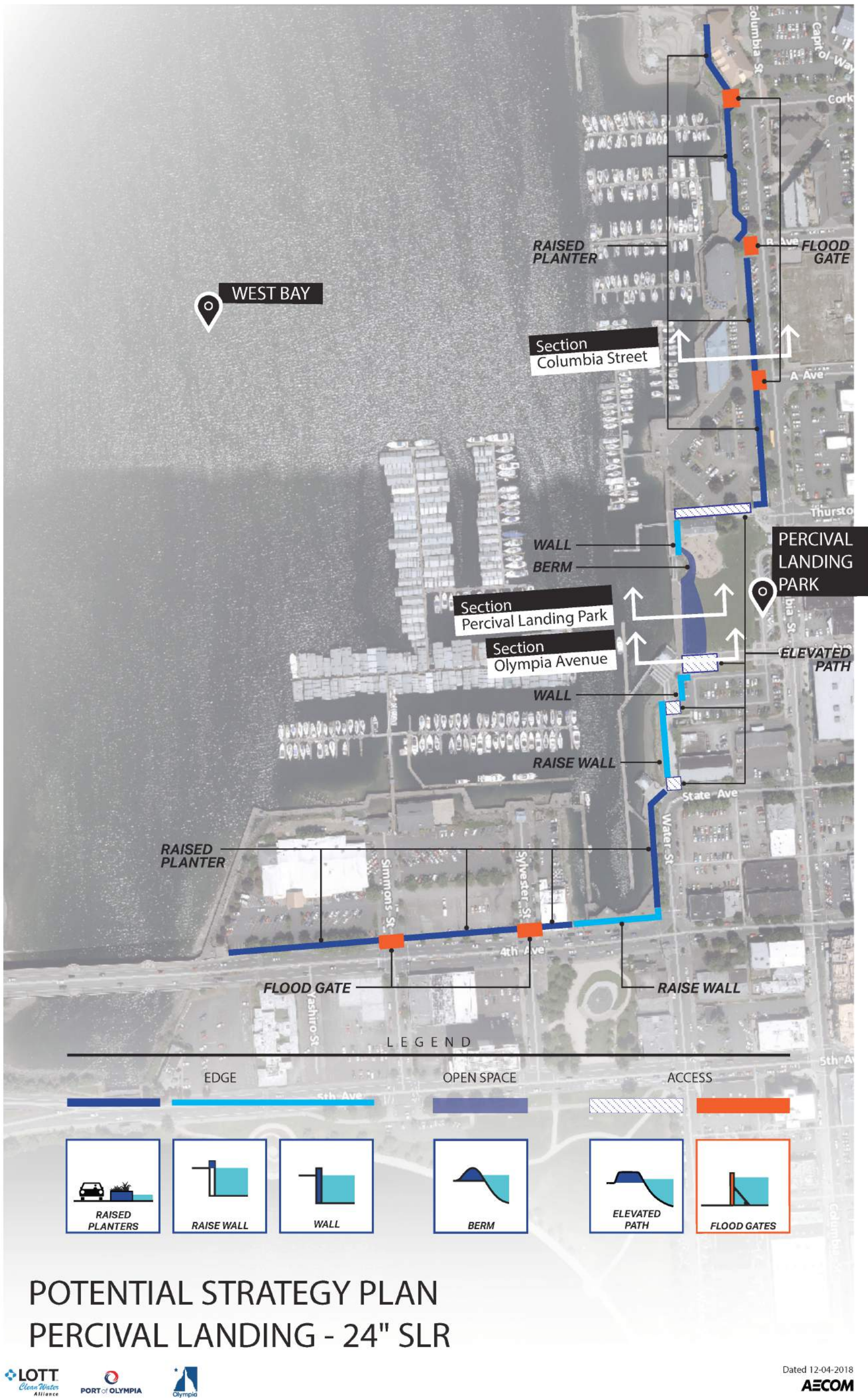
Figure 22. Potential Strategy Plan for Mid-Term Sea Level Rise (24 inches) at Percival Landing
